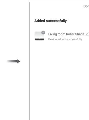
g. After the motor device is added successfully, the LED on motor head will be on for 10s and then go off.
